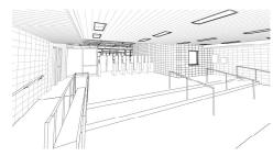
Customer Service Center office layout Removal of sloped floor and addition of stairs New ceiling and LED lighting
